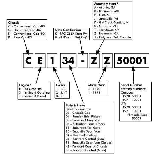
[1] When optional engines are available and selected, the Service Parts Identification plate would list the engine used. [2] List shown is applicable to Series 10-30 truck production only.
